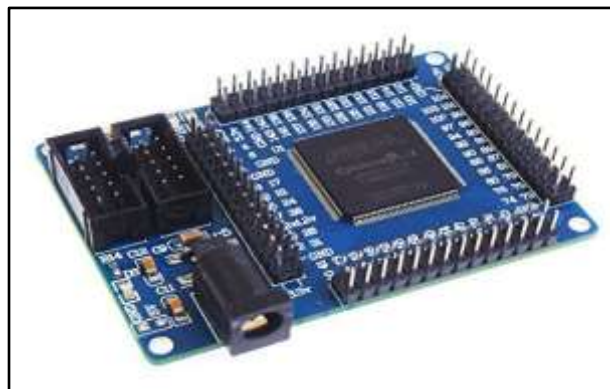
Figure 2. FPGA mounted on the card with peripherals
