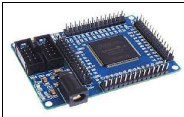
Figure 2. FPGA mounted on the card with peripherals
