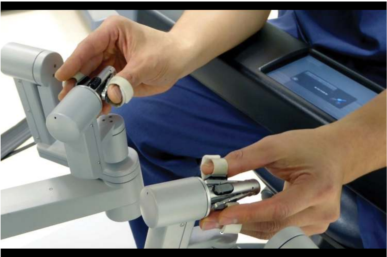
Figure 2. Controlling Robotic Arms with the da Vinci Surgeon's Console. Intuitive Surgical, Inc ® . Image available at: https://sius.davincisurgerycommunity.com/detail/videos/p9_rc_surgeon-console/video/5622753693001/instrument-controls:-using-the-masters?autoStart=true
