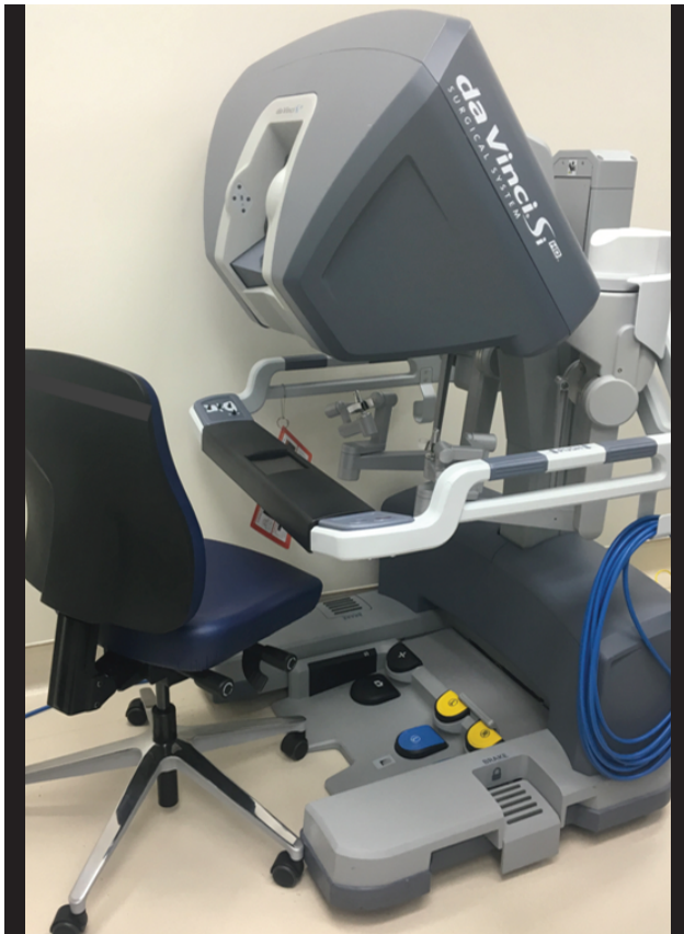
Figura 1. Surgeon Console in the da Vinci system.
